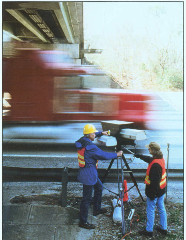
Determining whether vehicle occupancy is increasing -- and whether that is related to changes in air pollution -- will be easier using data collected by an infrared roadside camera GTRI researchers are developing.
