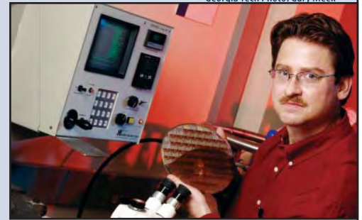
Professor John Cressler holds a 200 GHz silicon-germanium integrated circuit wafer at a cryogenic probe station capable of measuring temperatures to 200 degrees below zero Celsius.
