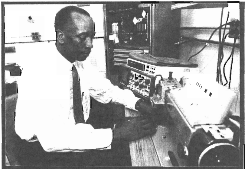
Bernard Gunn adjusts equipment used to measure acoustic energy produced by the needles of an industrial sewing machine. (Color/B&W Available).
