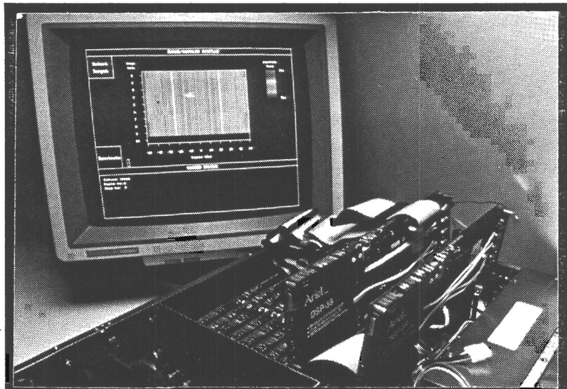
The Generic Doppler Processor could allow engineers to experiment with a variety of Doppler processing methods in real time using just one piece of hardware. (Color Slides/B&W Prints Available)
