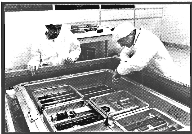
Dr. Don Blue and NASA's Dr. Jim Robertson examine a tray of electro-optic components exposed to space conditions aboard the Long Duration Exposure Facility (LDEF). (Color/B&W Available)
