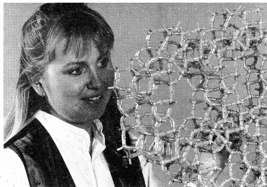
Kristin Sørby with a model of the large-pore molecular sieve she is using in her research on catalysts for producing gasoline from natural gas. (Photo by Joe Schwartz)
