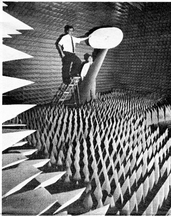
Gene Weaver (left) and Brian Shirley place a target on the new model tower in ECSL's fully automated compact range for antenna measurements in the 2-18 GHz region. (Photo by Gary Meek)
