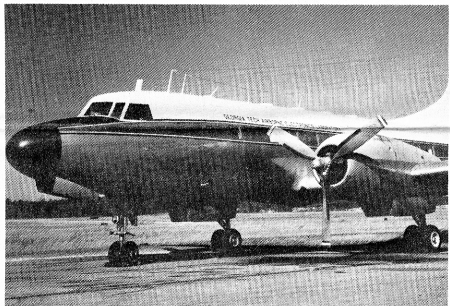
This is the T-29B (Convair 240), one of GTRI's two twin-engine, cargo type, pressurized aircraft which are used for flight testing of electronic equipment.
