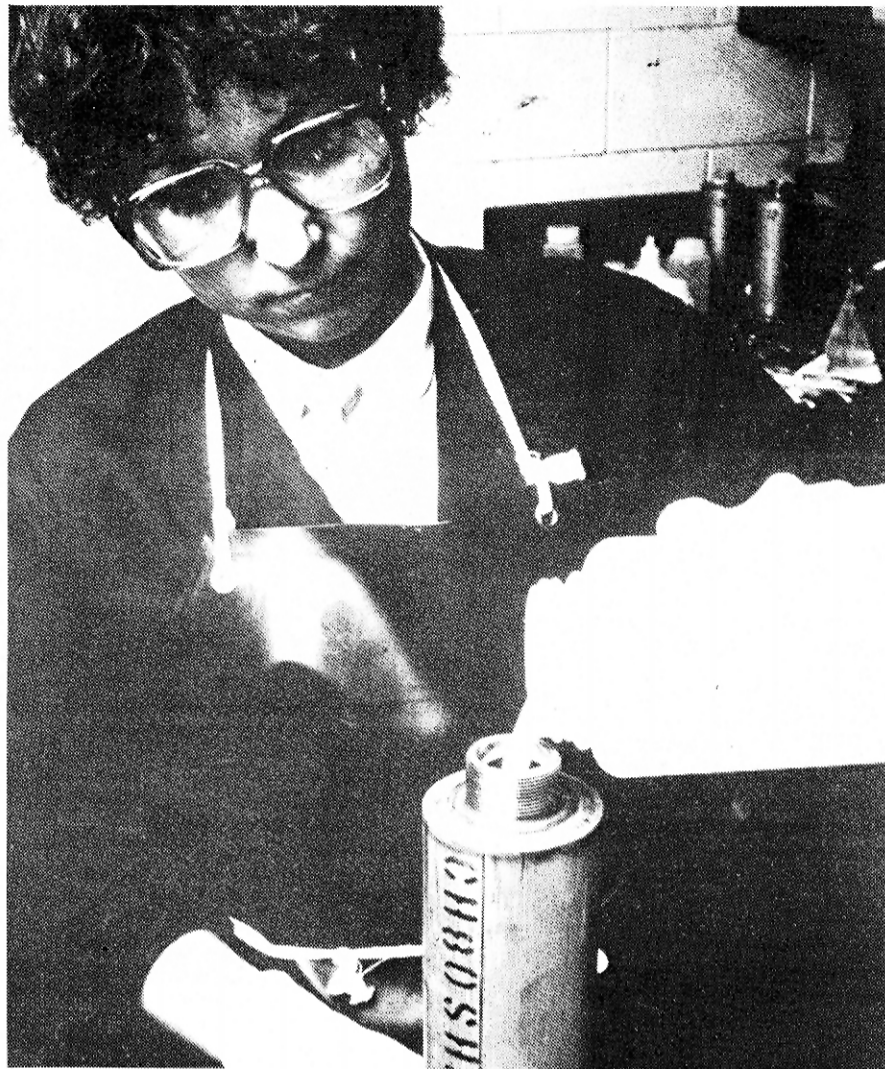
Rosemarie Szostak is pouring a gel mixture into a pressurized autoclave for synthesis into a new molecular sieve material. (Photo by Charles Haynes)
