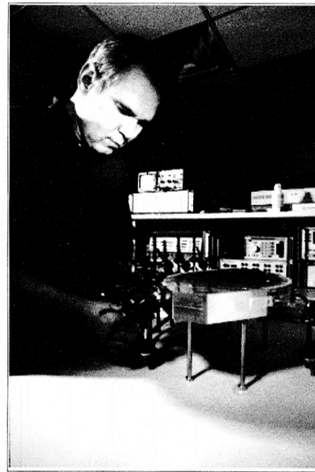
Otto Rausch attaches waveguides to prototype Rotman lens. (Photo by Stanley Leary)
