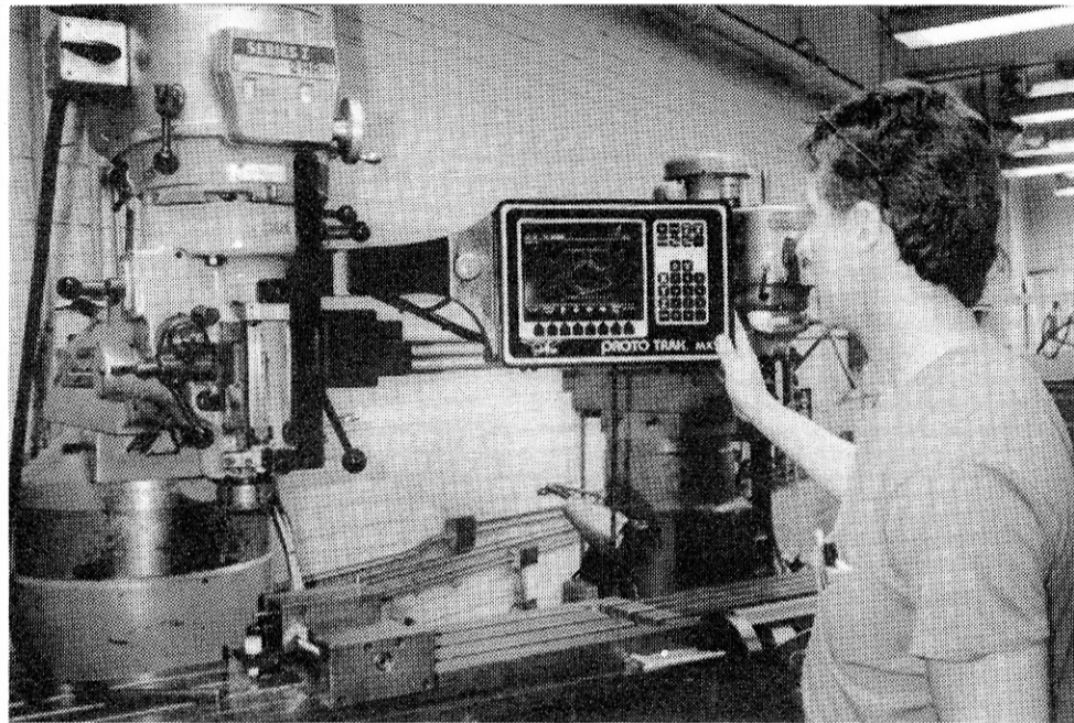
Randall Lloyd, Machine Shop, demonstrates a CNC 2 axis SWI Proto Trax MX2 retrofit on a Bridgeport Series I mills. The retrofit put the milling machine under computer control, offering new capabilities and making it 30 to 40 percent more efficient. (Photo by Lea McLees)
