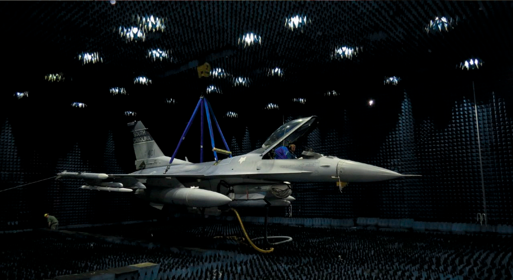
TOP: This photo shows a solar cell produced for space testing of new types of photovoltaic cell materials aboard the International Space Station. BOTTOM: GTRI's Josh Bosse supports F-16 radar warning receiver integration testing at the Eglin AFB JPRIMES Anechoic Facility.
