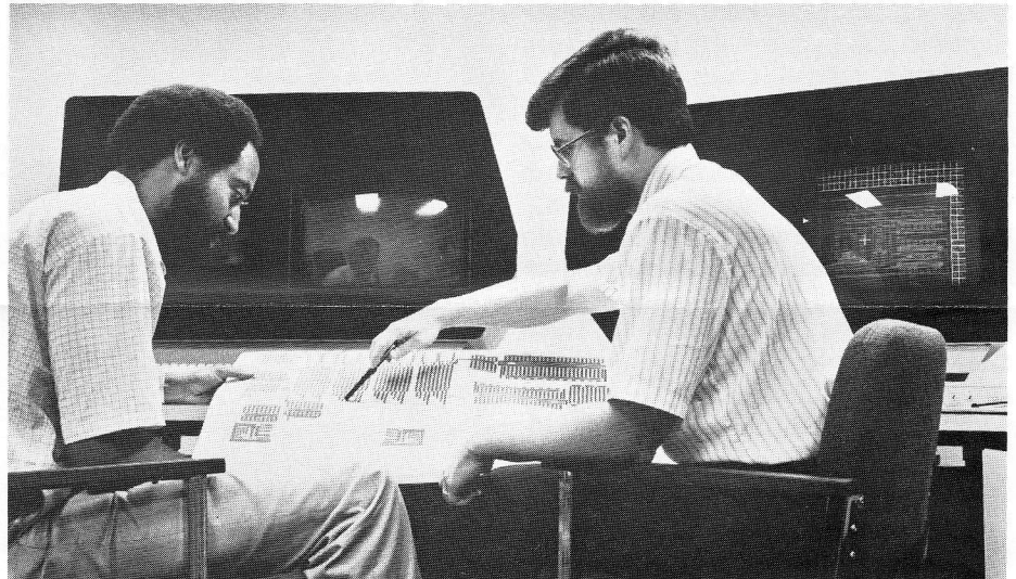
EES RESEARCHERS work at a CALMA CHIPS 220 Integrated Circuit Station. This high resolution color graphics system is used in laying out integrated circuits. Georgia Tech has purchased a CALMA unit which will be employed extensively in the Station's VLSI circuit design research.
