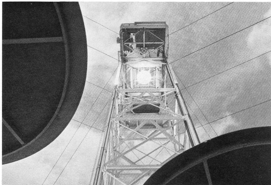
SUNLIGHT ILLUMINATES the focal point in the tower of the Department of Energy's 325 kW Advanced Components Test Facility at Georgia Tech. EES engineers will be using this receiver extensively in the operation of a major new solar energy R&D center at the Station.
