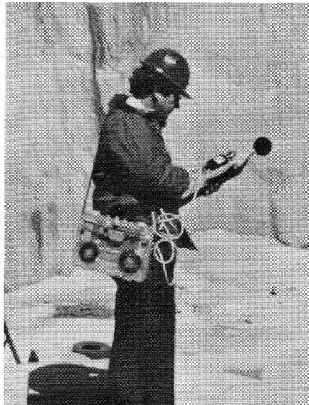
A staff engineer in EES' Industrial Extension Division performs a noise analysis test in a granite quarry near Macon. EES provides extensive assistance to Georgia industries with technical problems.
