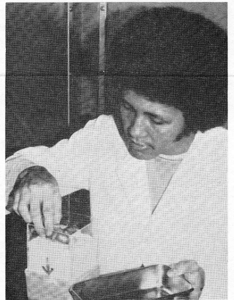
Electromagnetic radiation is used to thaw this dog kidney in experiments in Georgia Tech's Electronics Technology Laboratory.
