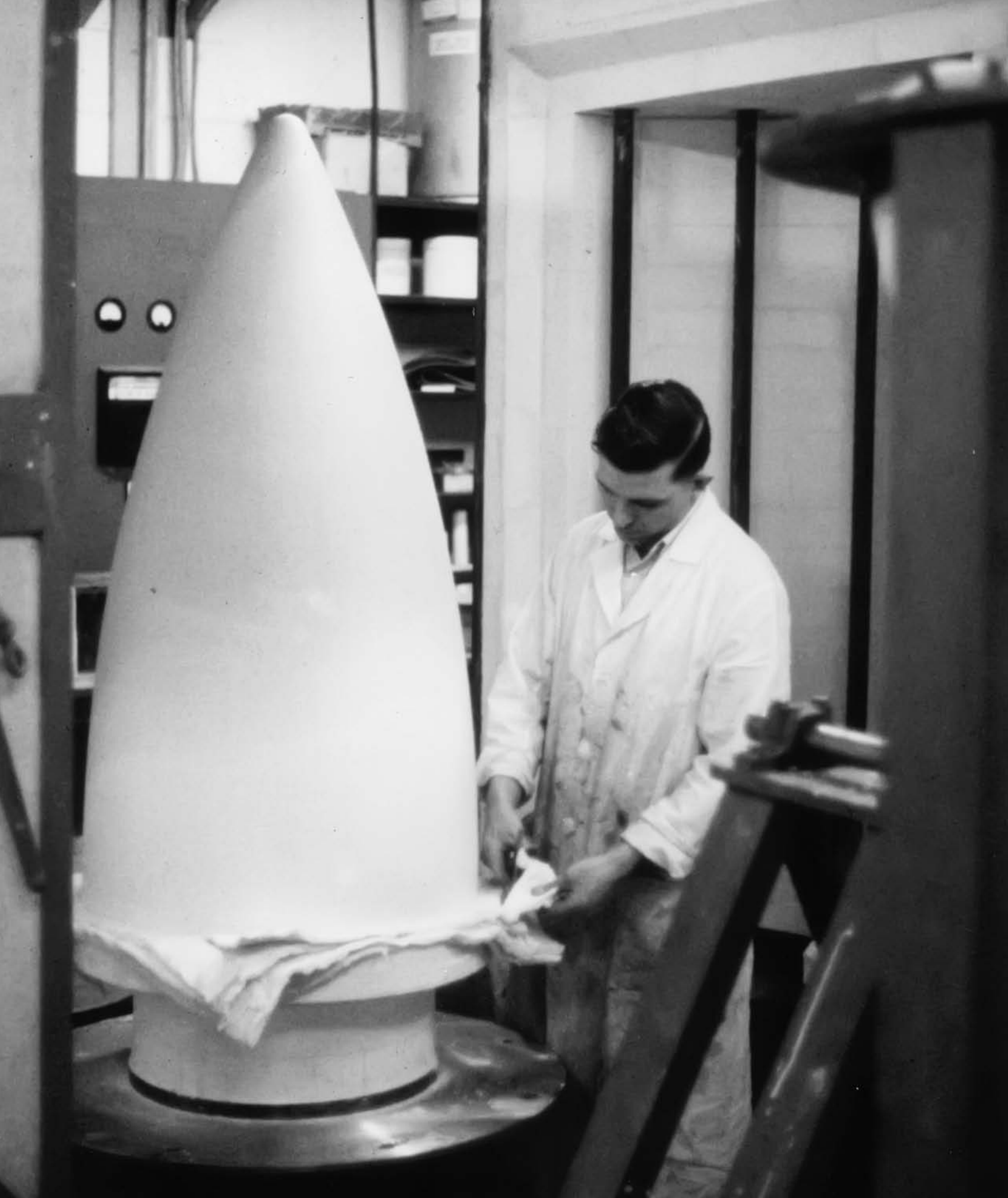
Expertise in high-temperature ceramics led the Engineering Experiment Station to develop a fused-silica technique for forming complex shapes such as missile radomes.
