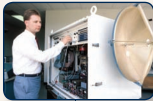
1980s – GTRI/EES work on millimeter-wave radar culminates in development of what was at the time the world's highest-frequency microwave radar, operating at 225 GHz.
