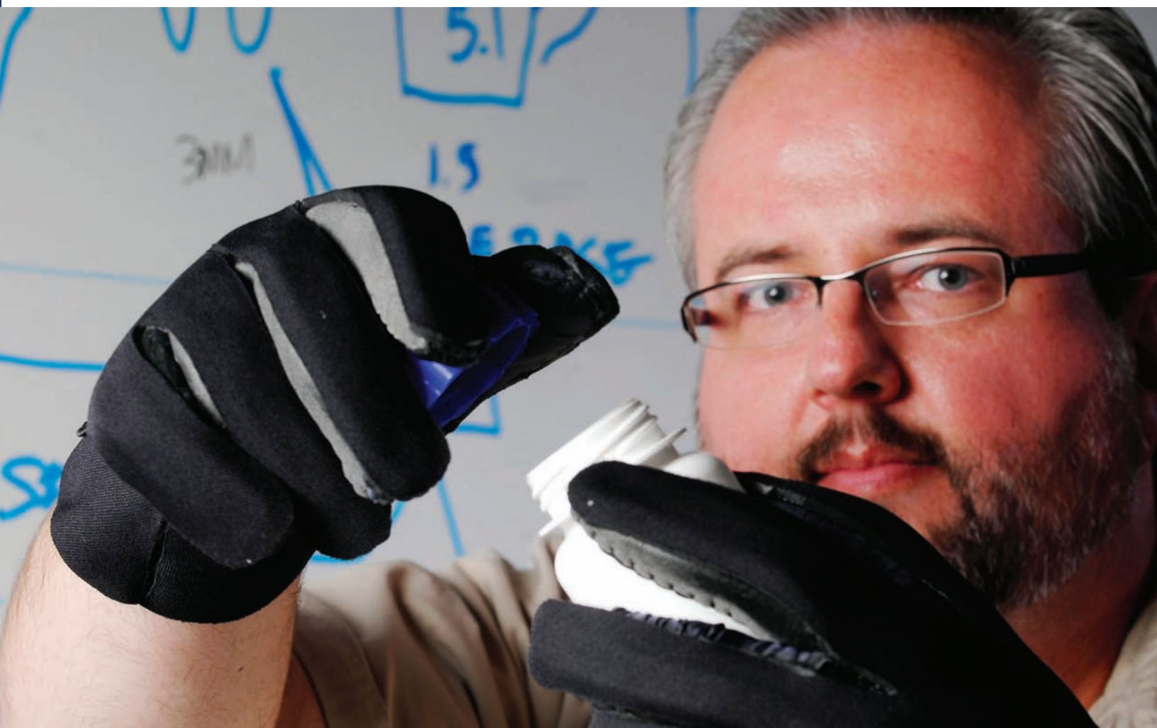
GTRI principal research scientist Brad Fain opens a medicine bottle while wearing the arthritis simulation gloves. The gloves reproduce the reduction in functional capacity experienced by persons with arthritis.
