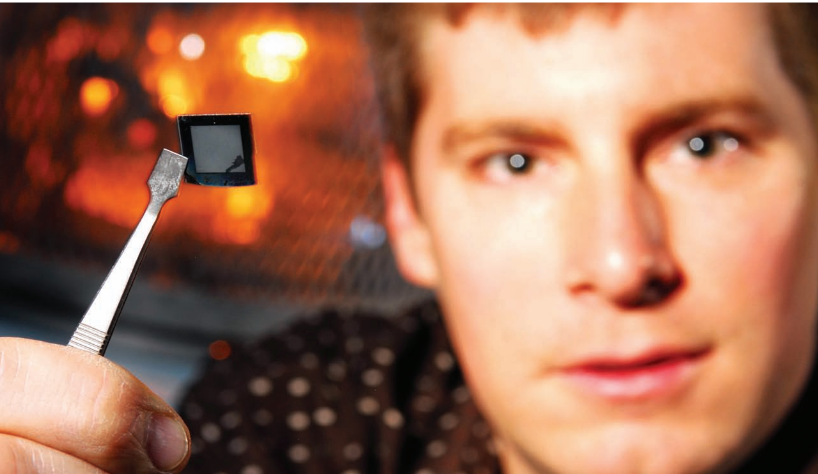
GTRI senior research engineer Jud Ready holds a sample of the 3-D solar cells developed to catch as much as three times as much light as flat solar cells.
