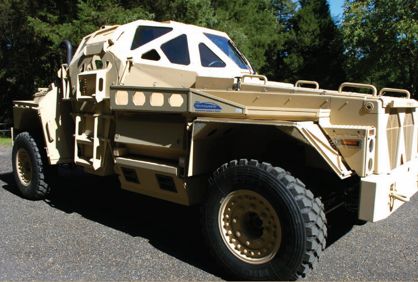
For the Office of Naval Research, GTRI created the ULTRA armored patrol vehicle to evaluate potential technology options for improving survivability in light armored vehicles. The concept vehicle combined advanced armor technologies with modern vehicle design and a diesel engine.
